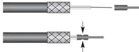
5. Recommended: Crimp a wiring tip (1 mm<sup>2</sup>, length 8 mm, red color)
