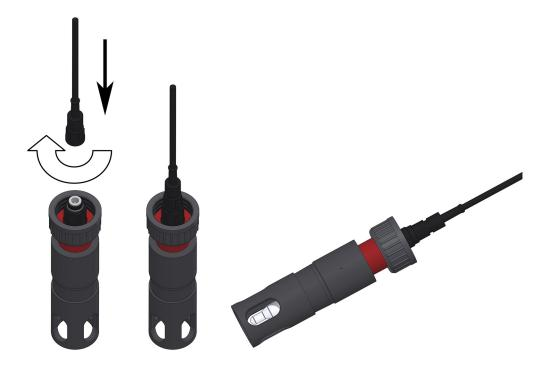
Pass the cable throug the head housing and screw the holder on the bottom of probe
