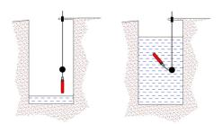
The NIVOSTOP SS2 is a float switch for level control in tanks and catch basins. The cigar-shaped version is designed for introduction in a tank through a small hole of  $\varnothing$  30 mm.
