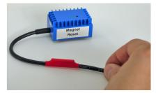
To perform the reset, lift the magnet, which is integrated in the cable and marked with a red shrink sleeving, onto the sticker with the inscription "MAGNET RESET".
