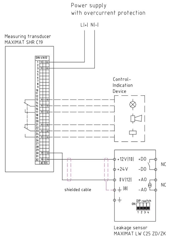
MAXIMAT LW C25 Z to MAXIMAT SHR C19 measuring transducer
