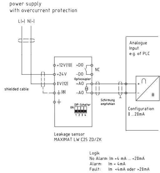
MAXIMAT LW C25 Z current output to PLC analogue input
