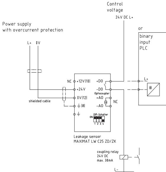
MAXIMAT LW C25 Z... binary output to coupling relay or PLC
