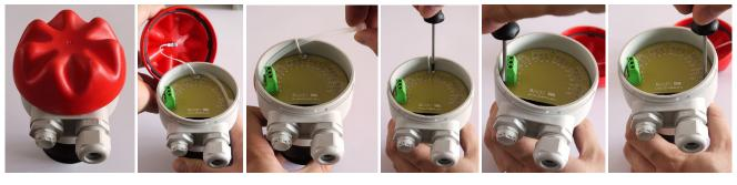
2. Feed the sensor cable from below into the connection head through the cable gland
