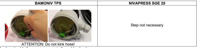
8. Insert cable for your process via the cable gland.
