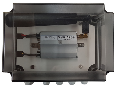
Modem mounted in IP67 case
